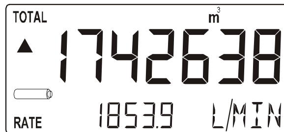
Fig. 4: Example of low-battery alarm
