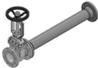
Valve partially closed upstream
