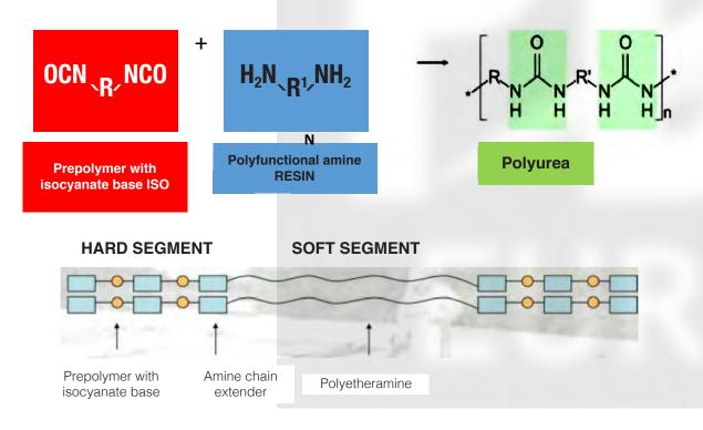
In aromatic systems, the isocyanate component is made from prepolymers based on methylene diphenyl diisocyanate (MDI); in aliphatic systems, from hexamethylene diisocyanate (HDI), isophorone diisocyanate (IPDI) or H12MDI methylene dicyclohexyl diisocyanate and it constitutes the hard segment of the chain.
