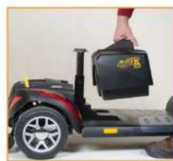
Step 2: Pull out the battery pack!
