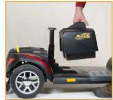
Step 2: Pull out the battery pack!
