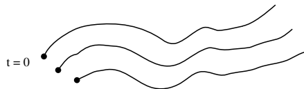
Fig. 2.1. Lagrangian description. Position of various fluid particles as a function of time.
