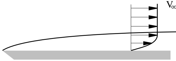
Fig. 12.2. Viscous boundary layer along a flat plate.
