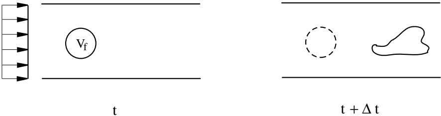
Fig. 5.1. Evolution of a fluid volume V_f(t) .
