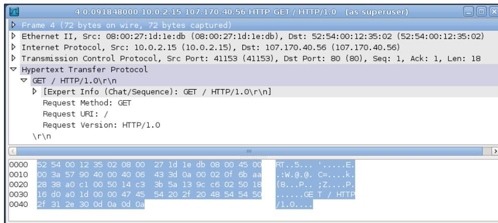
As you can see, the HTTP GET request has other components such as Request URI, version, and so on. Now you can check the HTTP response from the web server to your client. It has come after the TCP acknowledgment packet, that is, the sixth packet. Here, the server typically sends an HTTP response code (in this case 200), content length, and the data or web page content. The structure of this packet is shown in the following screenshot:
