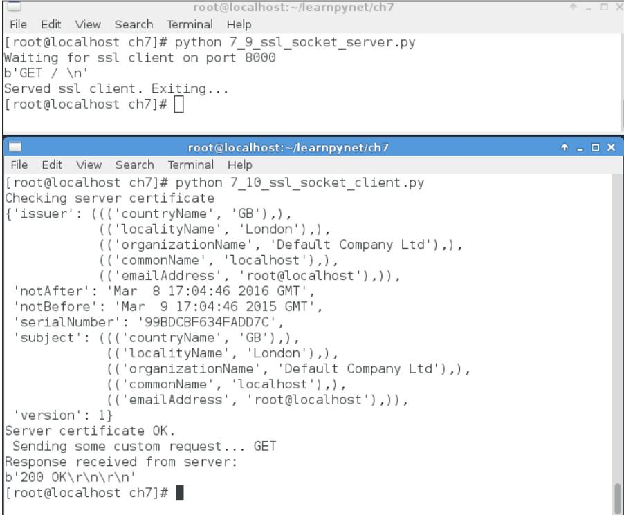
The image shows two terminal windows. The top window shows a server script (7\_9\_ssl\_socket\_server.py) that receives a GET request and prints the server certificate. The bottom window shows a client script (7\_10\_ssl\_socket\_client.py) that checks the server certificate, prints its details, and sends a GET request, receiving a 200 OK response.
