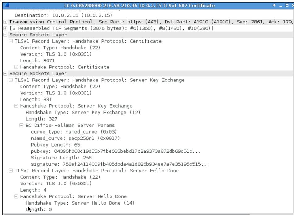
In the third phase of the handshake, the client exchanges a key and calculates a master secret to encrypt the messages and continue further communications. Client also sends the request to change the cipher specification that was agreed on the previous phase. It then indicates to start encrypting the message. The following screenshot shows this process:
