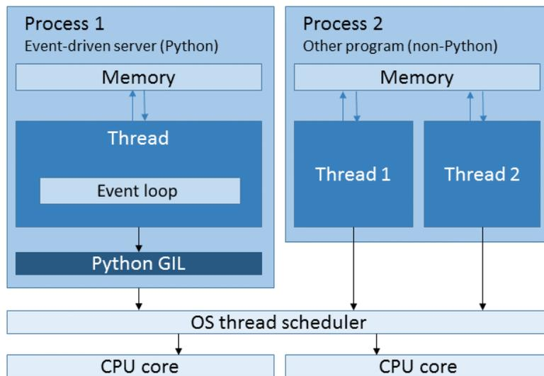
Although the GIL and the OS thread scheduler are shown here for completeness, in the case of an event-driven server, they have no impact on performance because the server only uses a single thread. The scheduling of I/O handling is done by the application.
