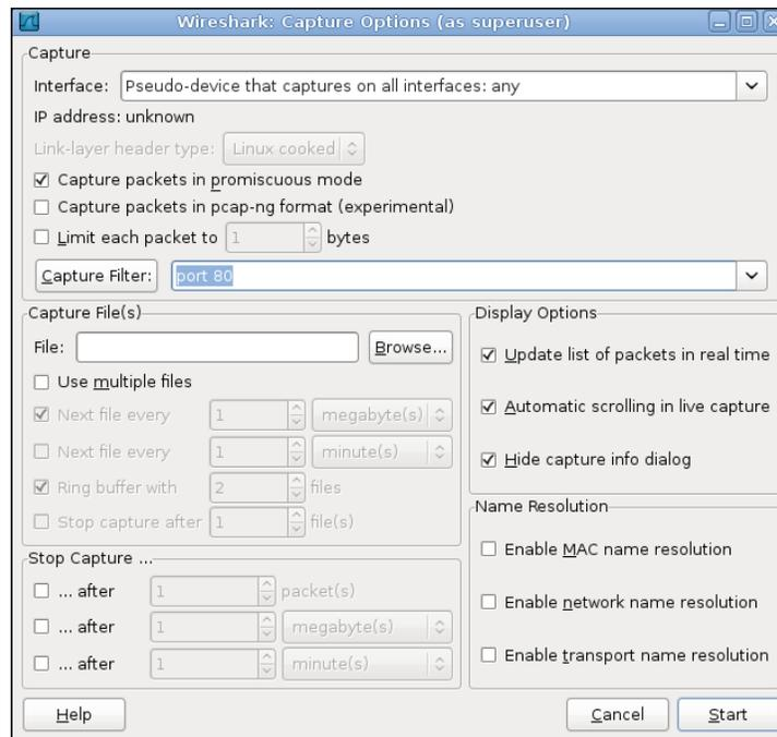
In the **Interface** option, we choose to capture packets passing through any interface. Now, if you run the preceding TCP client to connect to `www.linux.org`, you can see the sequence of packets exchanged in Wireshark, as shown in the following screenshot:
