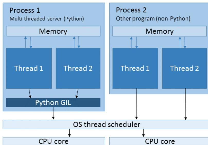
Threads exist within processes. A process can contain multiple threads but it always contains at least one thread, sometimes called the **main thread**. Threads within the same process share memory, so data transfer between threads is just a case of referencing the shared objects. Processes do not share memory, so other interfaces, such as files, sockets, or specially allocated areas of shared memory, must be used for transferring data between processes.
