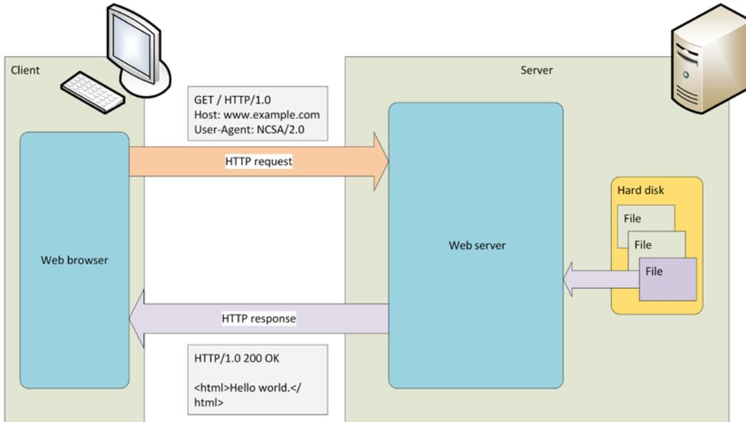
Here our web client sends an HTTP request to a server, where a web server program interprets the request, creates a suitable HTTP response, and sends it back. In this case, the response body is simply the contents of an HTML file read from, with the response headers added by the web server program.
