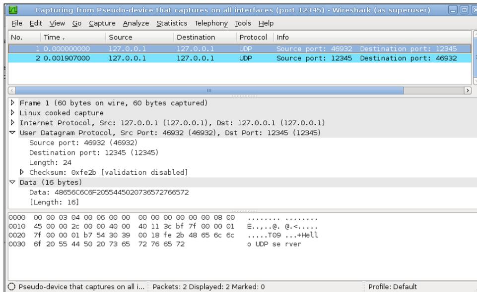
The following screenshot shows the server's response sent to the client. After inspecting UDP client/server packets, we can easily see that UDP is much simpler than TCP. It's often termed as a connectionless protocol as there is no acknowledgment or error checking involved.
