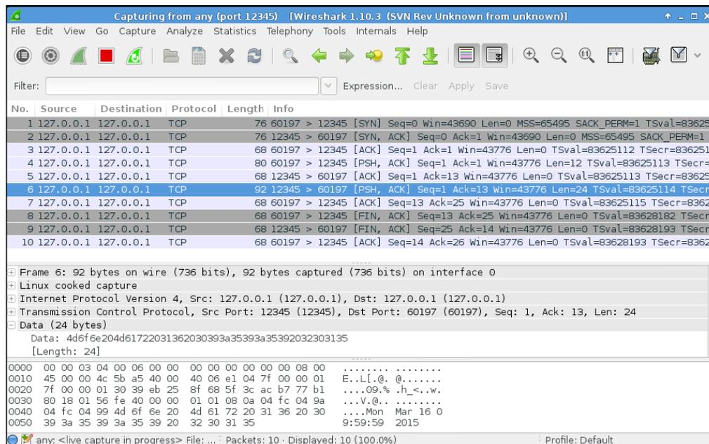
As we are capturing packets on a non-standard port, Wireshark doesn't decode it in the **Data** section (as shown in the middle pane of the preceding screenshot). However, you can see the decoded text on the bottom pane where the server's timestamp is shown on the right side.
