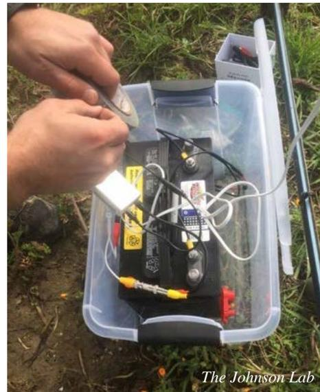
For longer studies, a system for recharging batteries should be established. If budgets and facilities permit, photovoltaic solar panels provide the lowest maintenance energy supply. However, if solar panels are not feasible, batteries must be replaced and recharged as needed. Many devices exist that use AC power to charge batteries and can be purchased for less than \$50 US.
