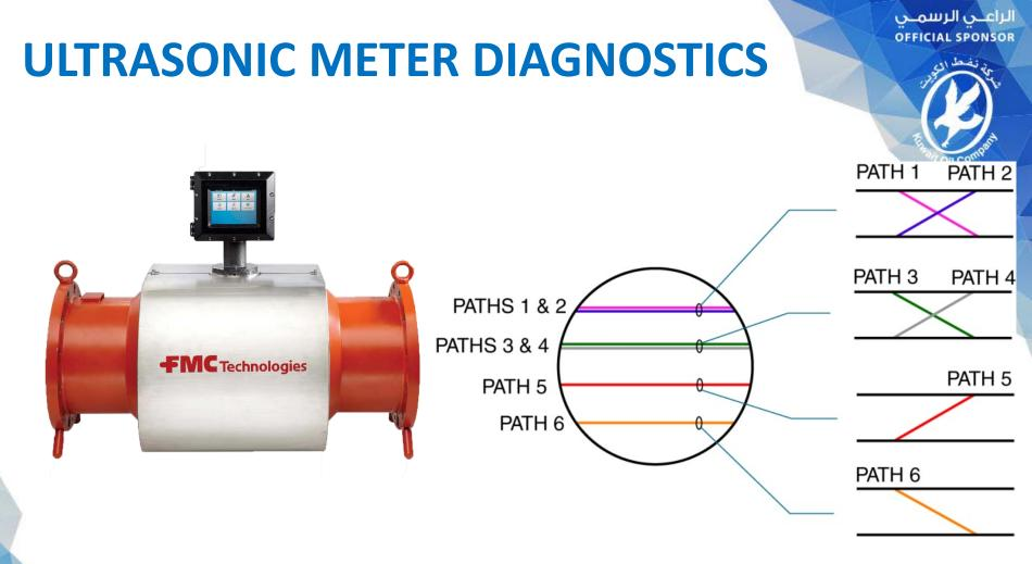
• Ultrasonic meters are **robust**, **reliable**, and have the ability to provide **custody transfer accuracy** over varied application ranges.
