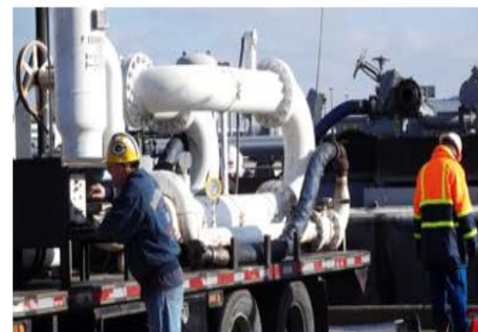
Proving of the Optimass 2000 S250
