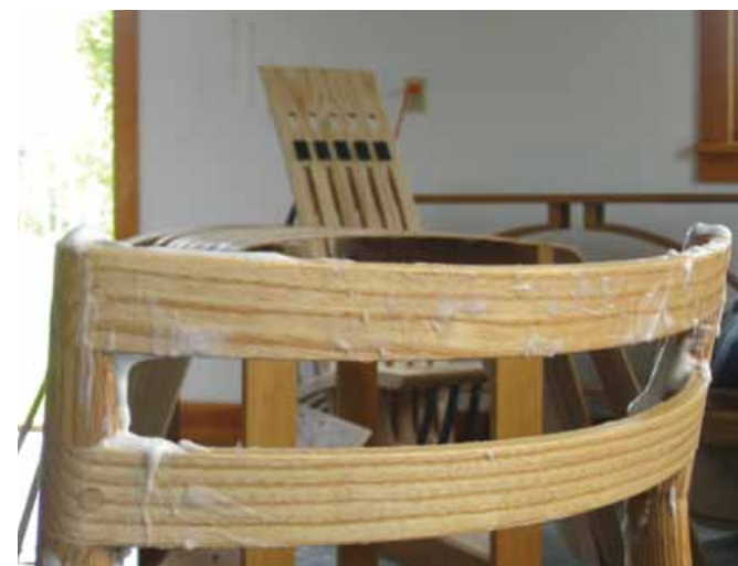
2 – Wet, Even Coats – Froth can be applied all over the piece, then left for a few minutes to soak in. Then use a clean cloth to remove any excess froth and wet areas from the finished piece. Once the piece is dry you can apply another coat.
